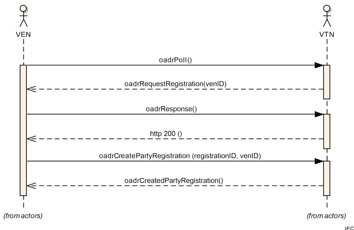
Figure 19 – Interaction diagram: oadrPoll (request reregistration reply)
