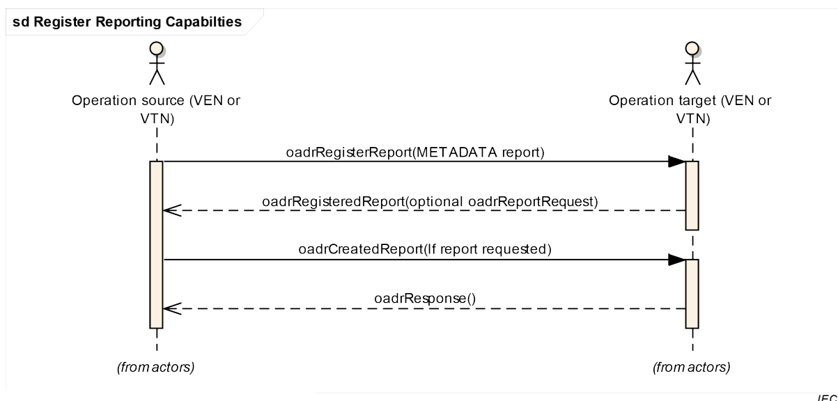
Figure 6 – Interaction diagram: Register reporting capabilities
