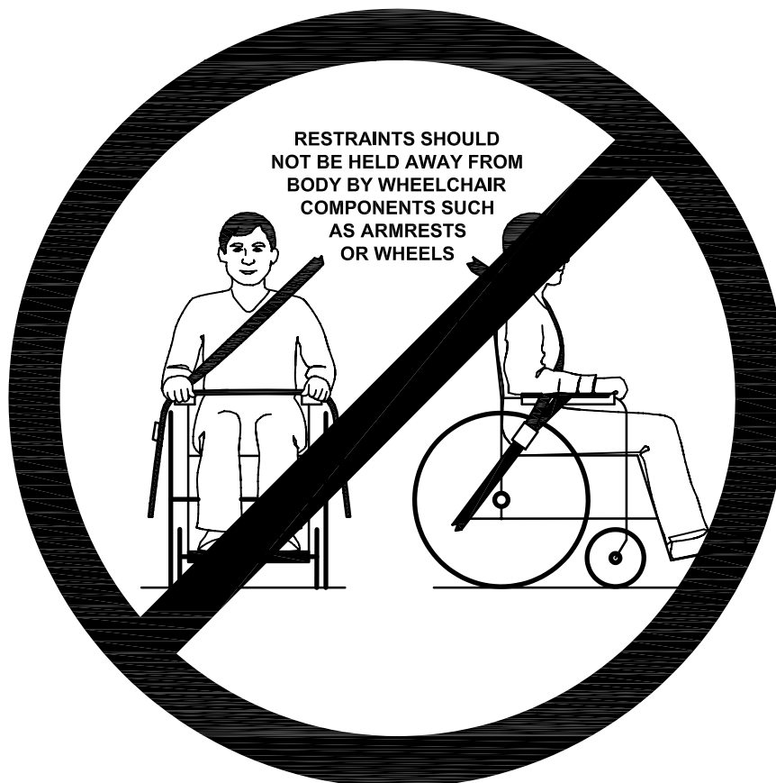
Figure 7 — Example of warning label illustrating improper positioning of occupant restraint belt
