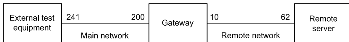
Figure 6 — Remote server system example 1
