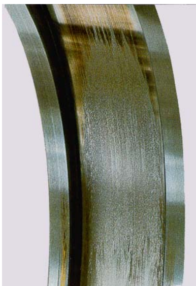
Figure 8 — Smearing on raceway surfaces
