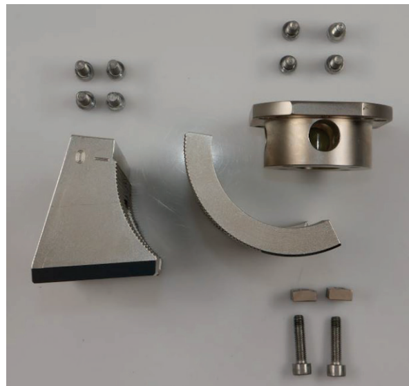
Figure A.12 — Separation of neck bracket assembly
