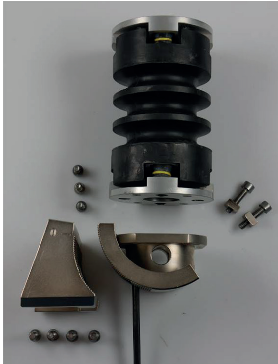
Figure A.9 — Removal of moulded neck from lower neck load cell structural replacement
