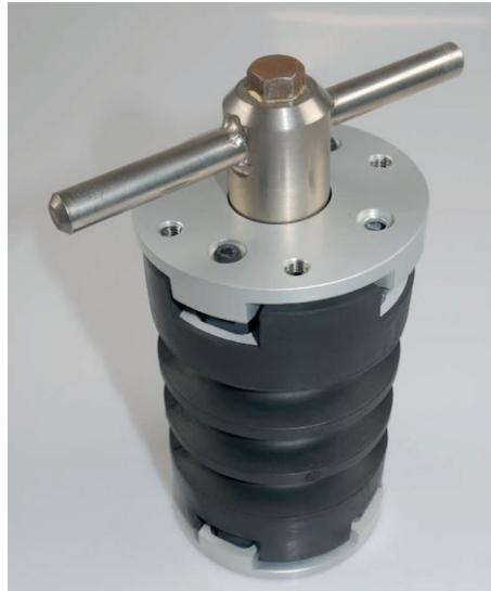
Figure A.11 — Removal of neck interface plates using neck compression tool
