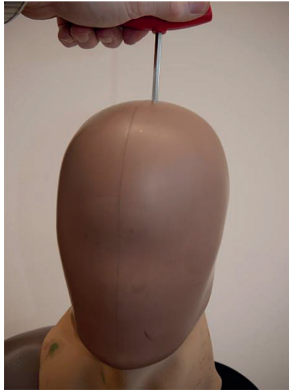
Figure A.3 — Removal of moulded head
