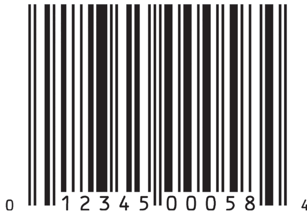
Figure 3 — UPC-A bar code symbol
