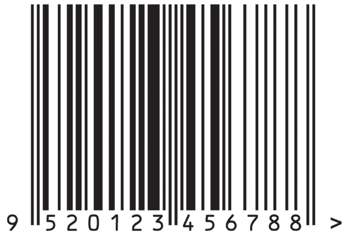
Figure 1 — EAN-13 bar code symbol
