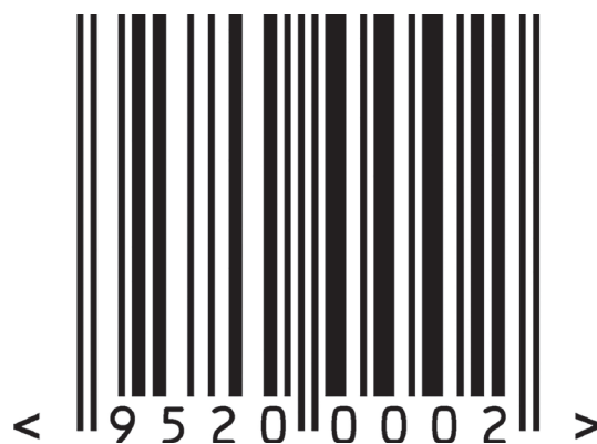
Figure 2 — EAN-8 bar code symbol
