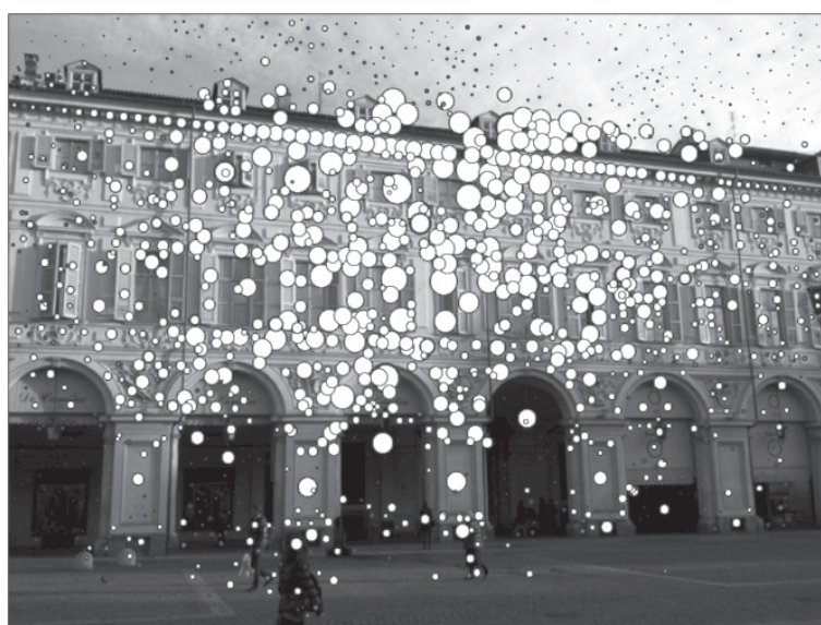
Figure 5 — The interest points of the image of Figure 4 plotted with circles whose diameters are proportional to the relevance measures
