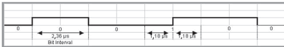
Figure 4 — Command MFM encoding and timing of binary 000100
