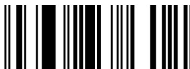
Figure 1 — GS1 DataBar Omnidirectional symbol representing (01)20012345678909
