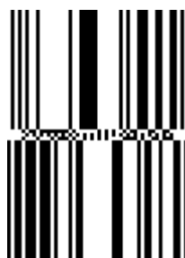
Figure 6 — GS1 DataBar Stacked Omnidirectional symbol representing (01)00034567890125
