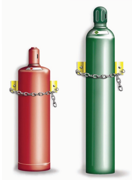
Figure 21—Securing Cylinders to a Wall
