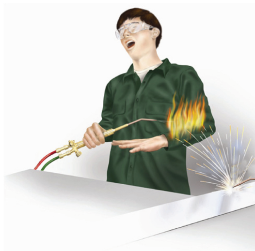
Figure 19—Oxygen from Welding Torch Blowing Dirt from Arm
