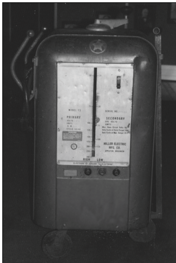
Figure 3—SMAW Power Source Used for Early Gas Tungsten Arc Welding
