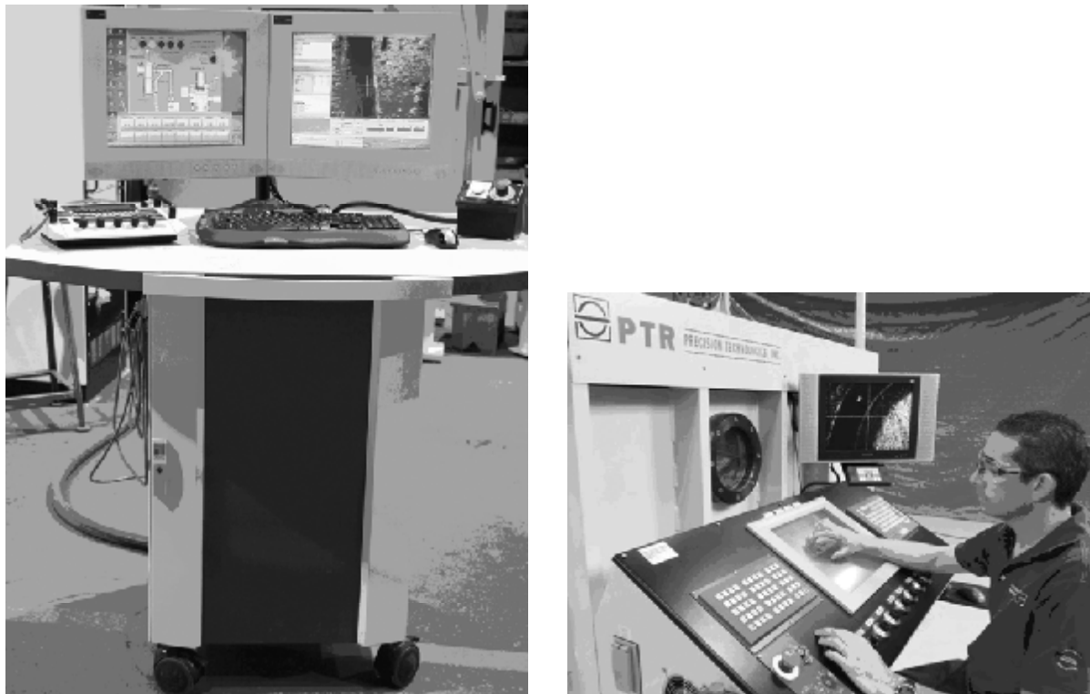
Figure 17—Electron Beam Welder CNC Pendant and Console
