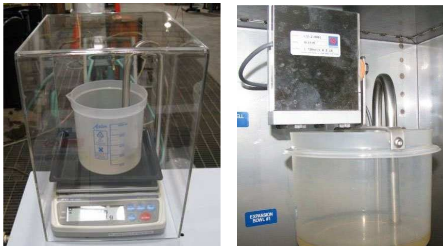
Figure 7—Typical nonburette EID systems
