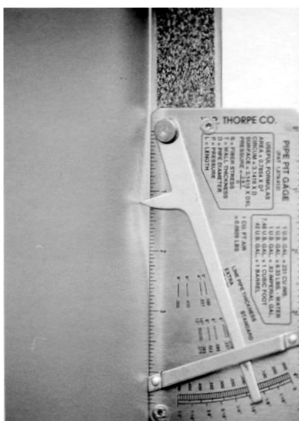
Figure 7—Measuring the length of a dent
