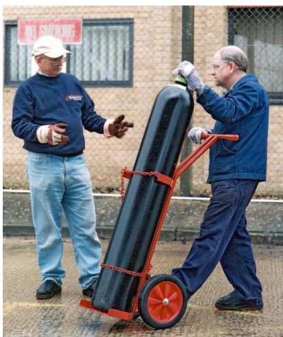
Moving compressed gas cylinder with assistance
