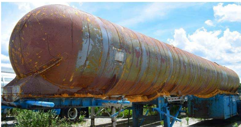
Figure 1—Example of trailer with insulation removed
