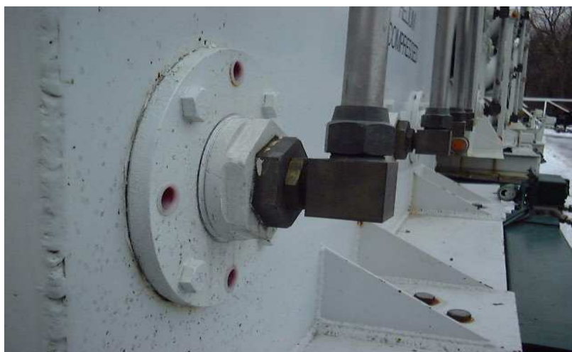
Figure 1—Pressure relief device assembly for the front end of a tube trailer
