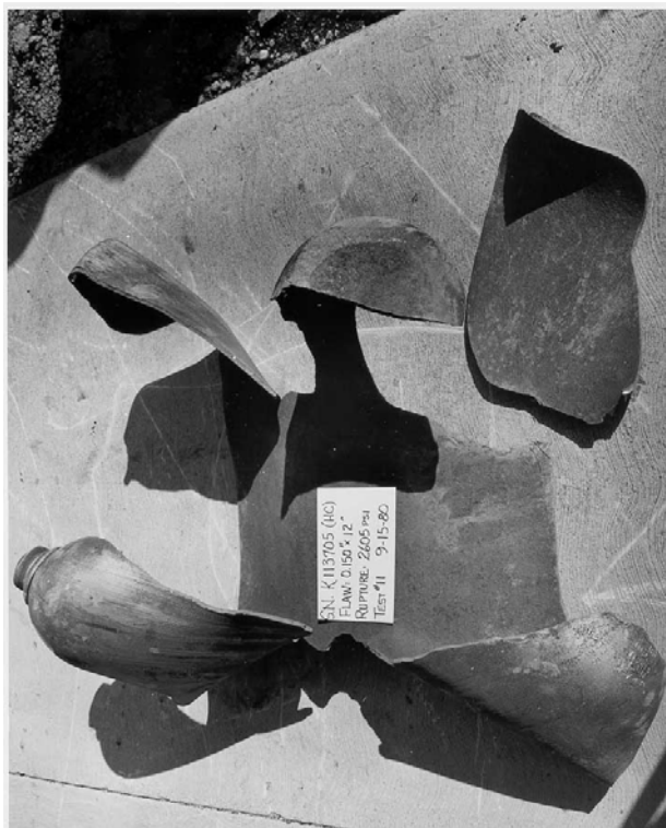
Figure 6—Flawed tested 3A cylinder (no. 4)
