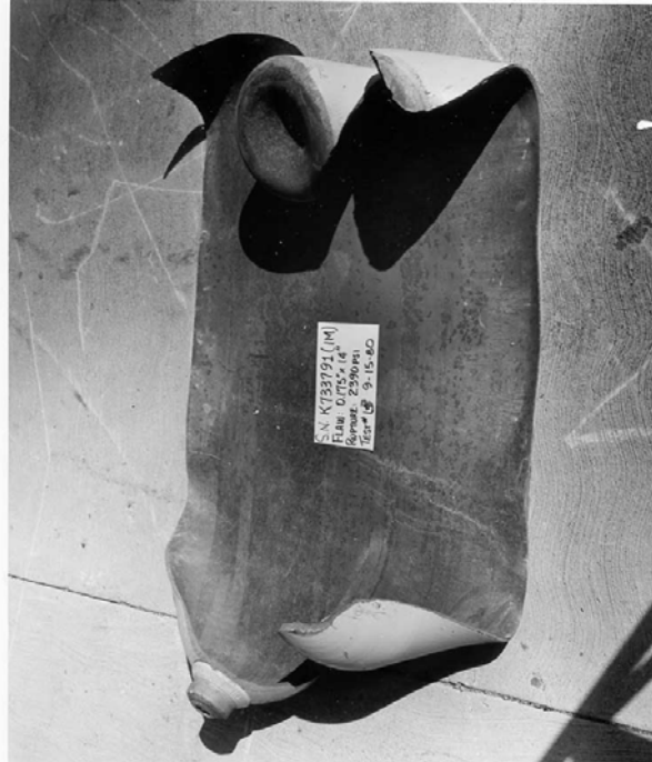
Figure 4—Flawed tested 3A cylinder (no. 2)
