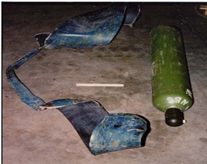
Figure 1—DOT-3AA cylinder in-service ruptured
