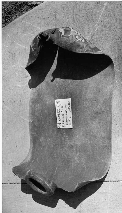
Figure 3—Flawed tested 3A cylinder (no. 1)
