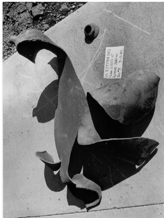
Figure 5—Flawed tested 3A cylinder (no. 3)
