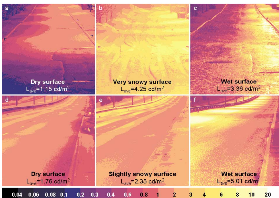
Figure 2. Luminance measurement results from a local street illuminated by HPS lamps under a) dry, b) very snowy, and c) wet weather conditions and from a highway illuminated by HPS lamps under d) dry, e) slightly snowy, and f) wet weather conditions (Ekrias et al., 2007).
