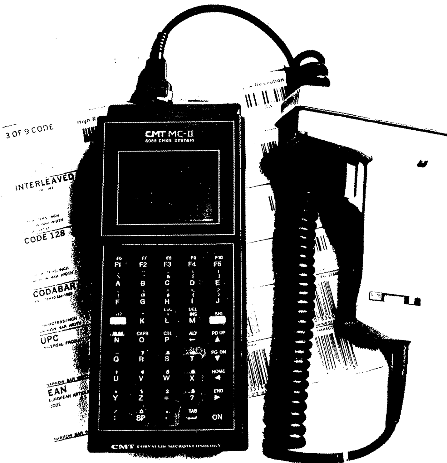
Figure 2-2. Portable Data Terminal (PDT) with Laser Gun Attached
