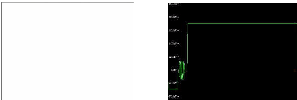
Figure 10: 100 IRE white field test pattern and associated waveform
