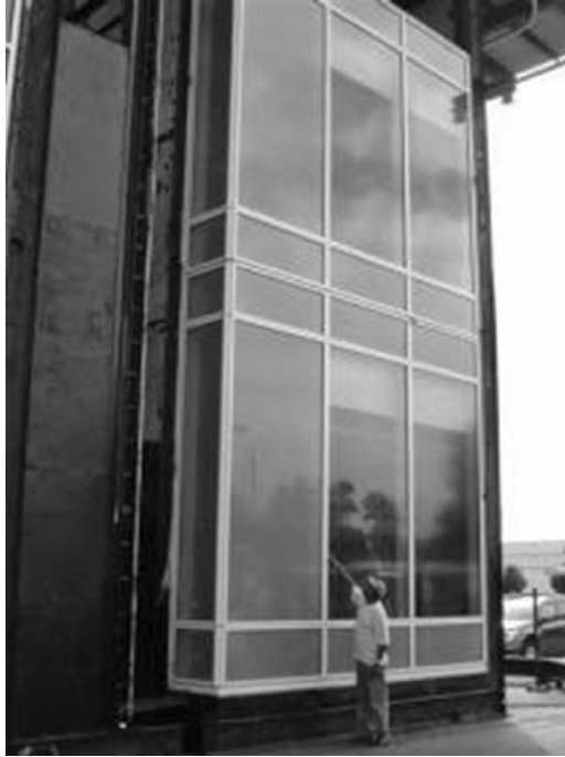
Fig. 4-3. Example of an installed two-story mockup for testing Source: Courtesy of Construction Consulting International; reproduced with permission
