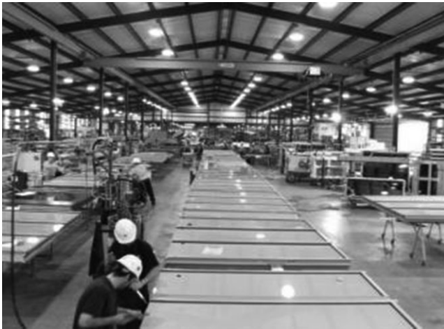
Fig. 3-15. Unitized or shop-assembled system
