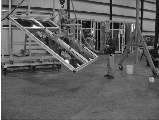
Fig. 3-16. Unitized or shop-assembled system
