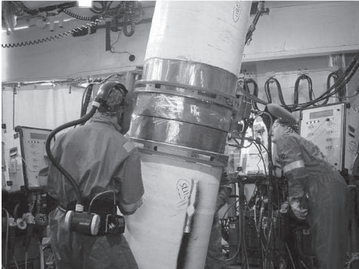
Figure 4—Typical Orbital Machine Pipe Groove Welding System Performing Offshore J-Lay Pipe Welding
