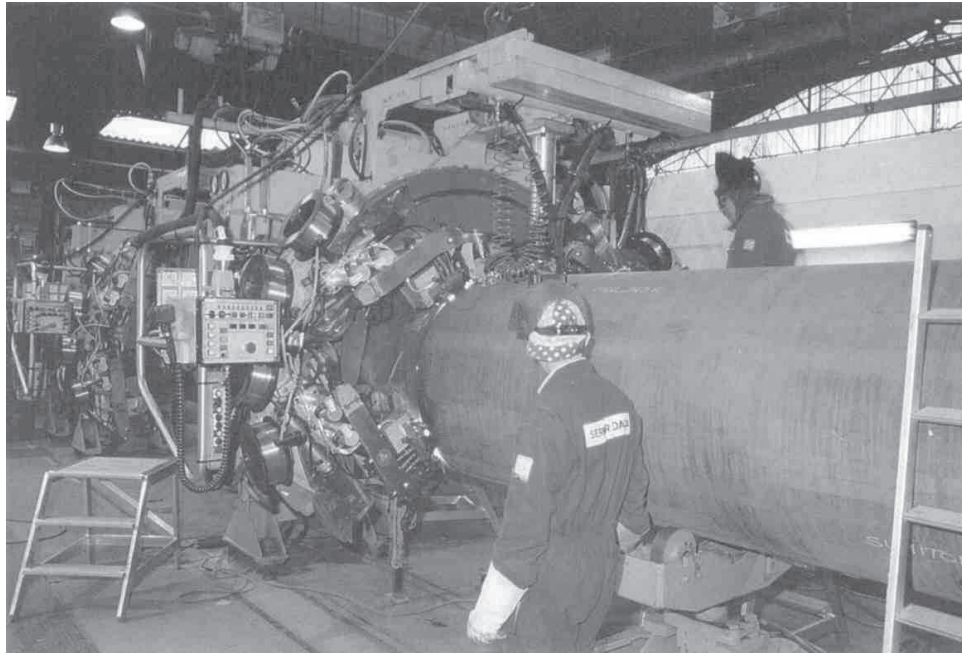
Figure 1—Typical Orbital Machine Pipe Groove Welding Clamshell Head
