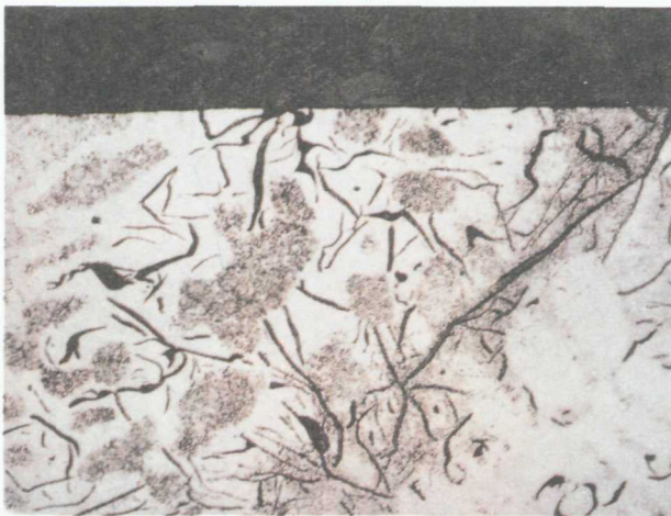
Figure 15 — Photomicrograph of HAZ Weld Toe Crack Shown in Figure 14 (Unetched, 15x Magnification)
