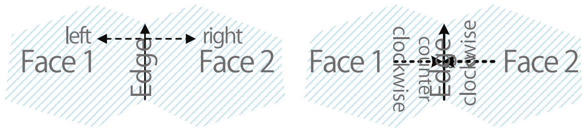
Figure 4 — Relation between Faces and bounding Edges
