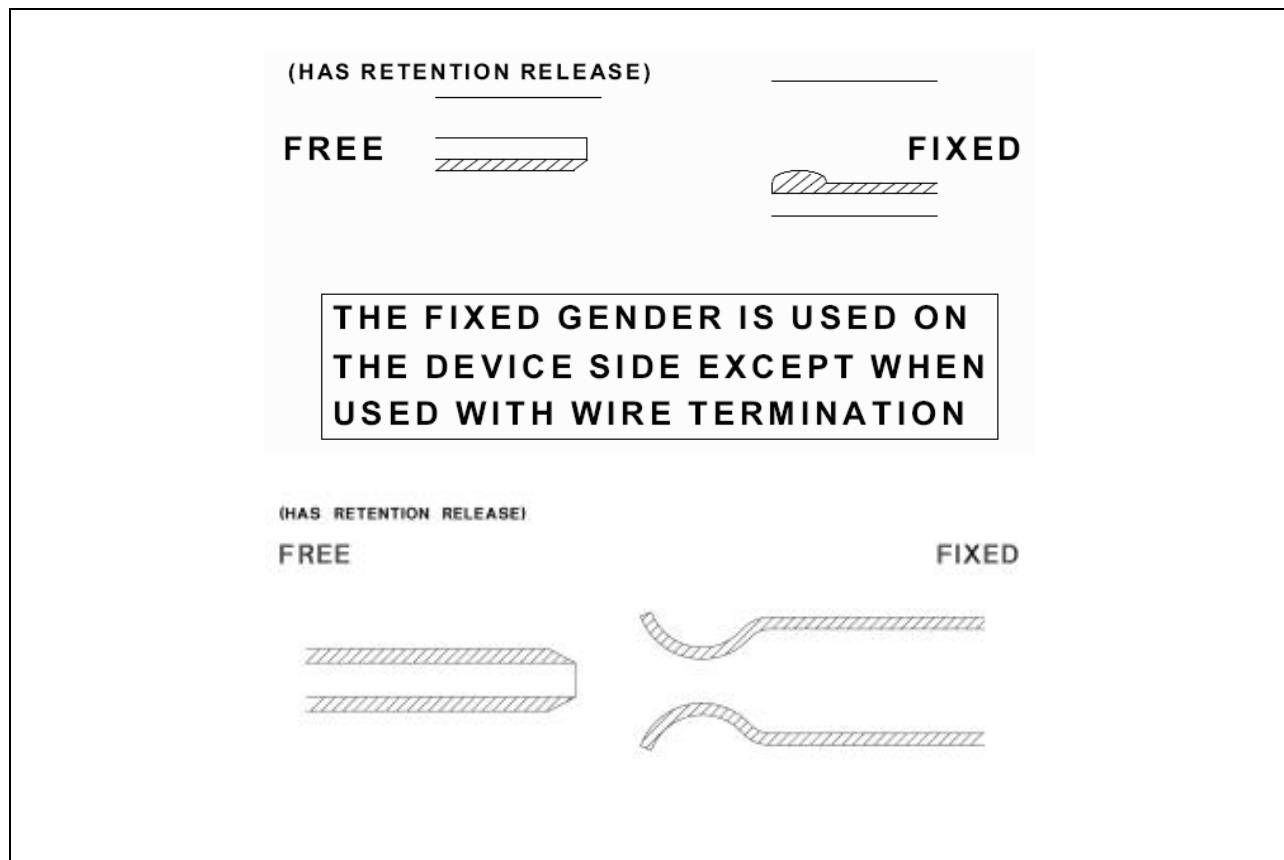
Figure 3.1- Mating side gender definition
