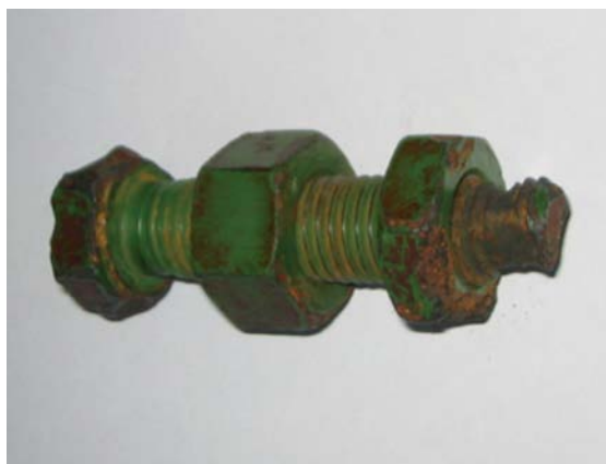
Figure 2 PTFE coated subsea fastener
