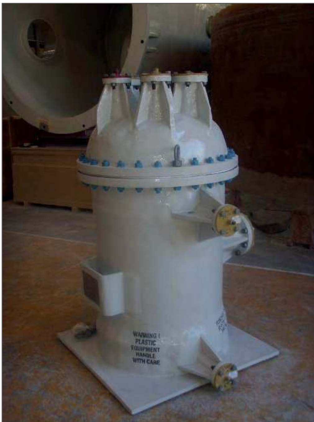
Figure 3: GRP tank showing outlets
