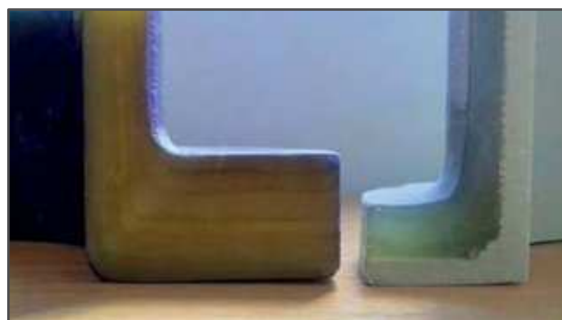
Figure 10: GRP and lined-GRP flange sections
