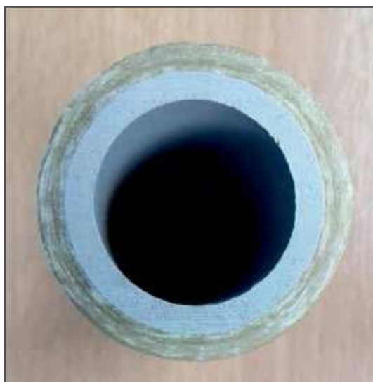
Figure 12: Lined GRP pipe section
