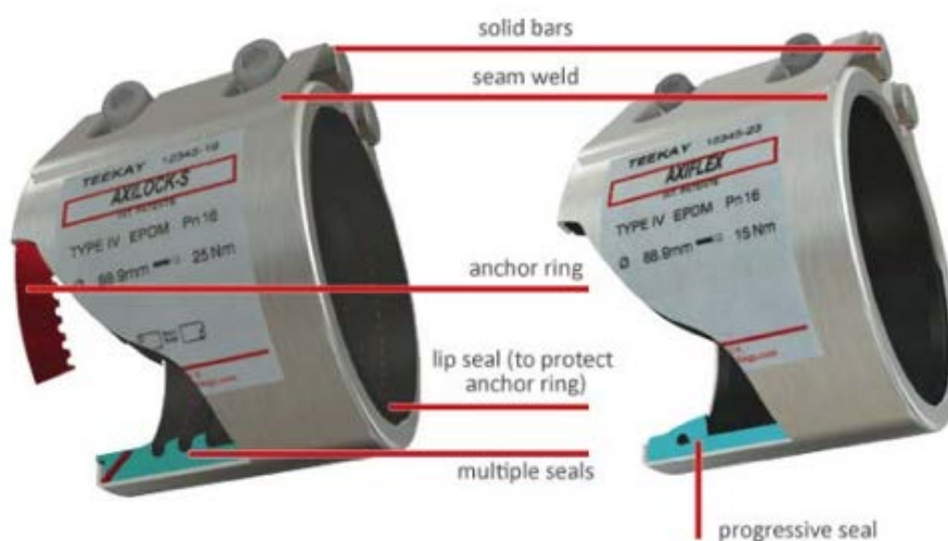
Figure 6 – Axial Grip & Non-Grip Type Couplings
