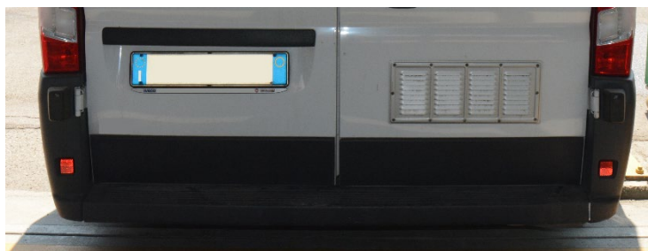
Figure 1 Typical ventilation grill at the bottom of the rear door on delivery vehicle
