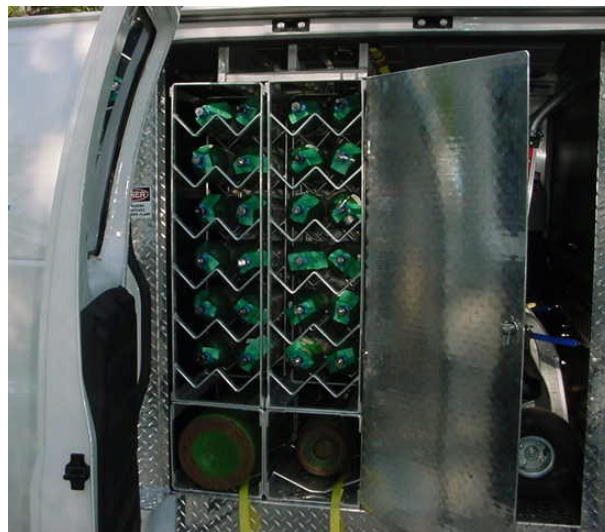
Figure 2 Typical cylinder storage rack on delivery vehicle
