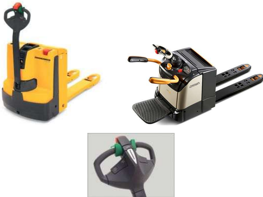
Figure 4 Typical pallet truck, platform pallet truck and controls
