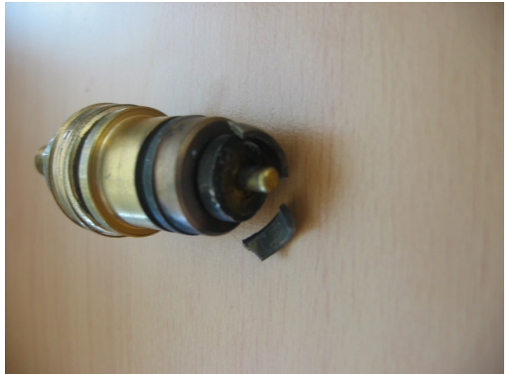
Figure 1: broken lower spindle seal retention skirt
