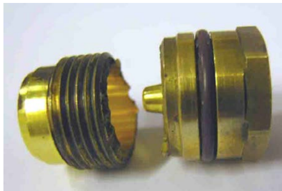
Figure 3: defective residual pressure valve plug
