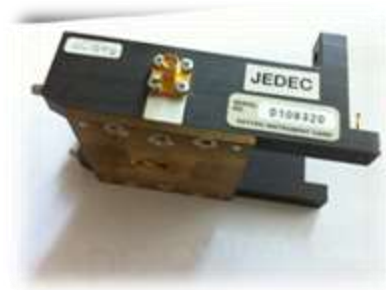
Figure 6: JEDEC CDM Test Head used for Current Measurements in the Field
