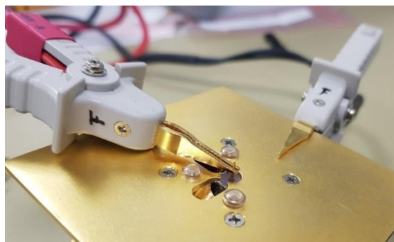
Figure 3b: Connection of the Kelvin 4-Wire Clips to the 1-Ohm Current Sensing Resistor Setup
