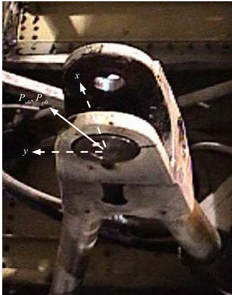
A typical lug under oblique load (Airbus A300 rudder hinge lug)
