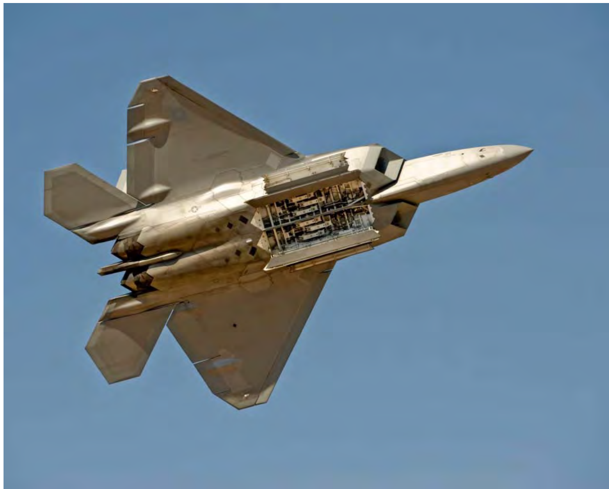
Sketch 3.1 Lockheed Martin F22: Bay doors showing serrated (sawtooth) edges (Photo © Tom Dowd, Dreamstime.com)
