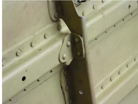
Structural cleat – illustrating the principle of fitting a minimum of two attachments per face
