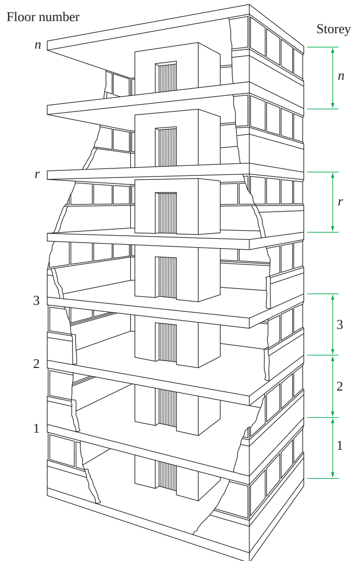
Sketch 2.1 Typical core building structure
