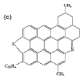
Figure 1. Planar (2D) structures of model asphalters and resins. (a) Model BC5, 2 stable continental asphaltene from a Venezuelan crude oil. MW: 1003, formula: C_{50}H_{16} . (b) Model CO2, 21 unstable continental asphaltene from a Venezuelan crude oil. MW 1208, formula: C_{50}H_{12}NO_{1.5} . (c) Model asphaltene from a Mayan crude oil. 22 MW: 794, formula: C_{37}H_{10}NS . (d) Model archipelago asphaltene. 23 MW 1653, formula: C_{118}H_{31}NOS_2 . (e) Model resin from an Athabasca sand oil. 19 MW 194, formula: C_{17}H_{14}S . (f) Model resin from an Athabasca sand oil. 19 MW 320, formula: C_{15}H_{14}O .
