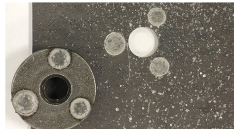
Figure 3 – Interfacial Fracture Example
