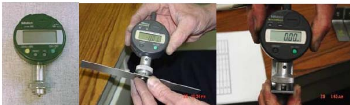
Flushness Gauge (To calibrate the gauge place on a surface plate feet down and press the zero button)
