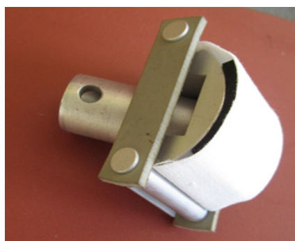
1b: Micro-scratch head in assembled condition with lapping film.
