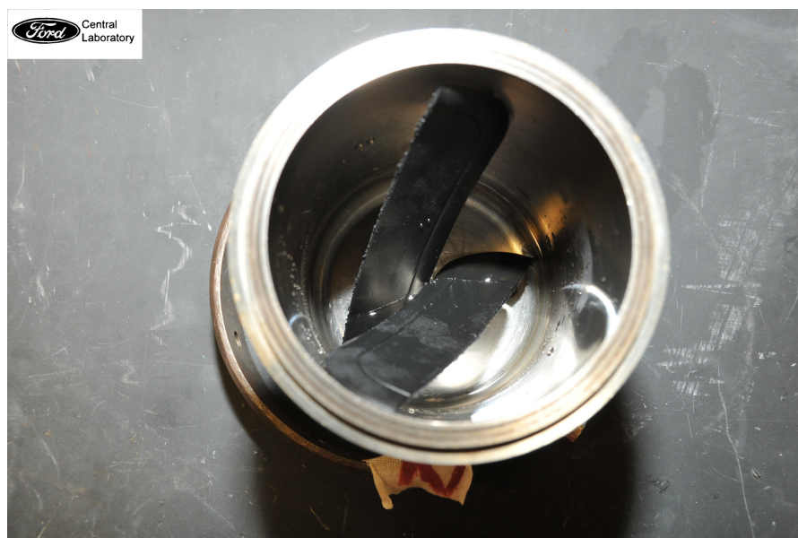
Figure 1: Body plug in pressure vessel with synthetic exhaust condensate.
