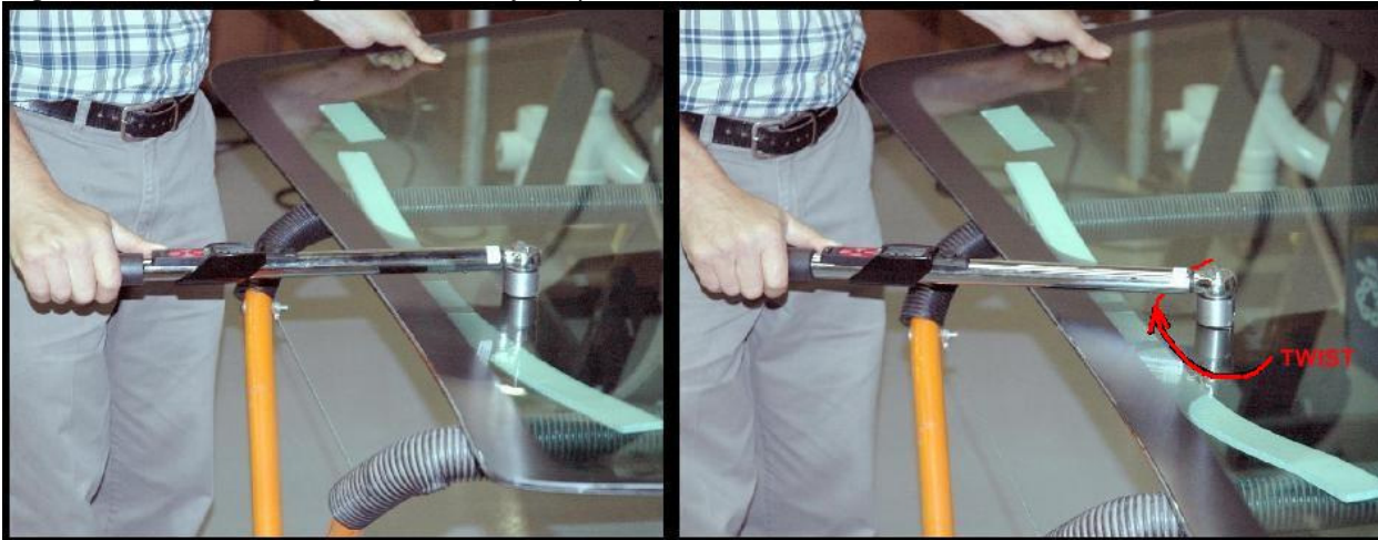
Figure #3 – Determining the breakaway torque on a full windshield
