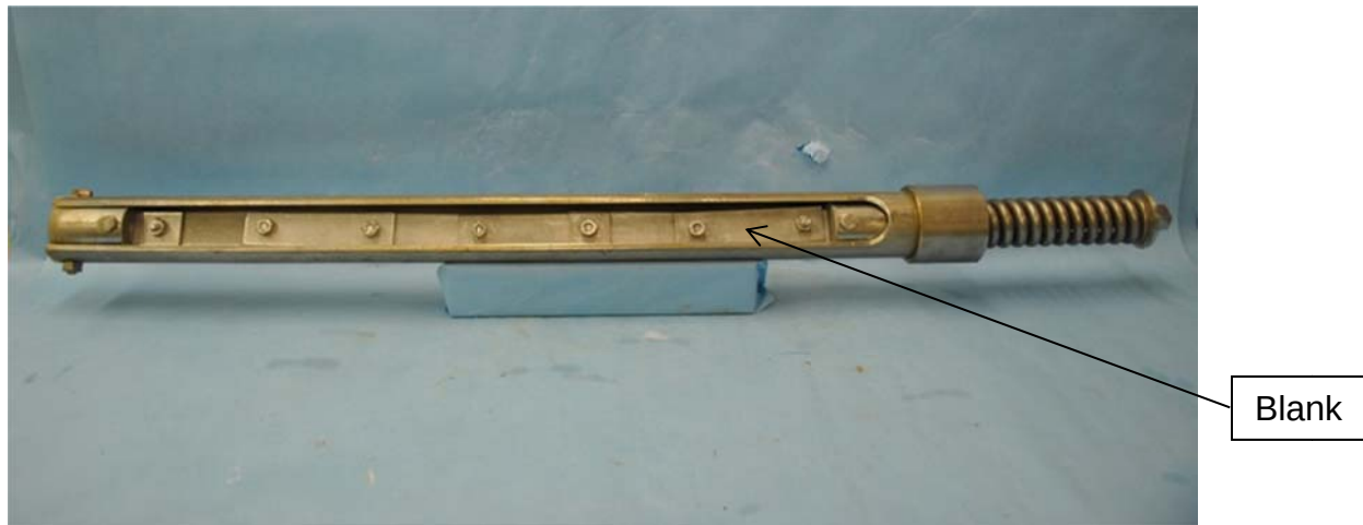
Figure 1: Stress Durability Fixture Assembly with Blanks
