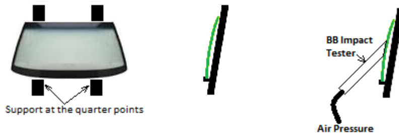
Figure 1 - Stone impact test support at the quarter points.
