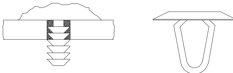
Figure 1 -- Typical Fir Tree, Bayonet and Other Push-in Type Features
