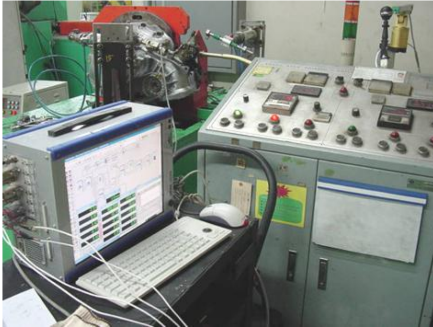
Photo 1: Test Equipment of Reverse Shift Performance /
