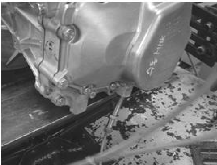
Photo 2: RPM Measurement Part - Gap Sensor /
