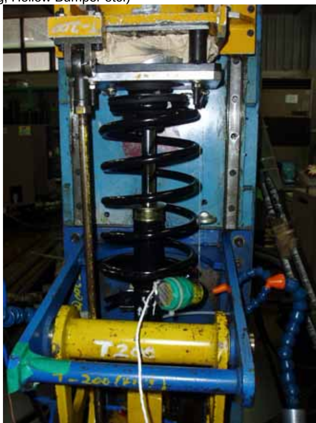
Fig 1. Strut System Test Rig
