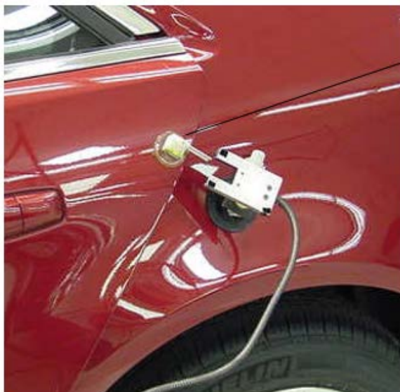
Figure 1: Velocity Meter Positioning
